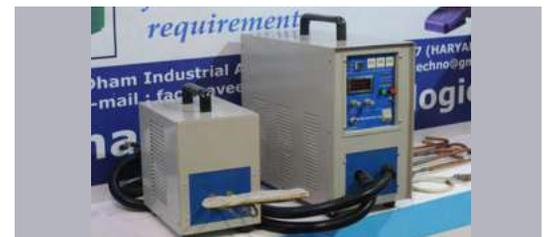
Induction heating machine incorporate high frequency generators for non-contact heating of metal using electromagnetic induction.
