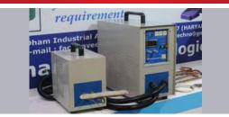
Induction heating machine incorporate high frequency generators for non-contact heating of metal using electromagnetic induction.
